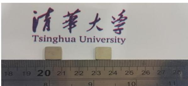
Fig. 2 TCA samples without silver micro-flakes (left) and with silver micro-flakes (right)
